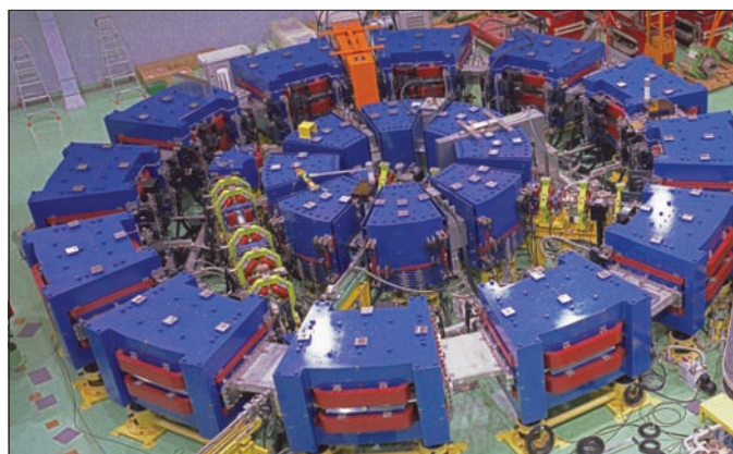
Fig. 1. The proton FFAG accelerator developed at Kyoto University Research Reactor Institute (KURRI), Japan, for a basic experiment on accelerator-driven systems. A third injector ring is located outside this image frame. (Courtesy KURRI.)
